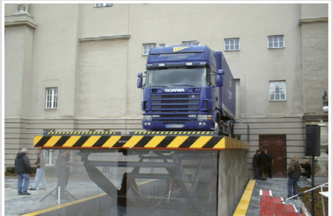
Platform lift with a 14.0 m x 4.5 m platform, Capacity 25 t
