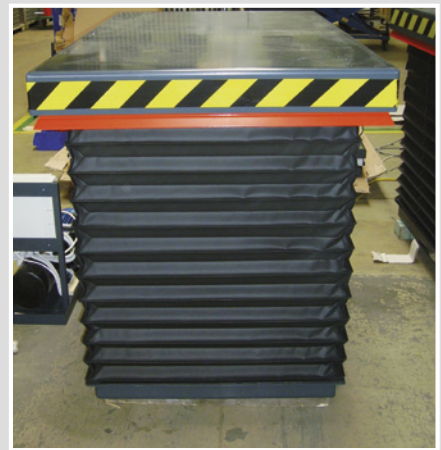
Capacity: 6.000 kg Bellows all the way round
