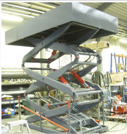
Capacity: 3.000 kg Effective Stroke 5.650 mm
