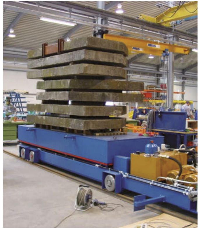
Capacity: 16.000 kg, Stroke 2.850 mm Carriage with geared motor
