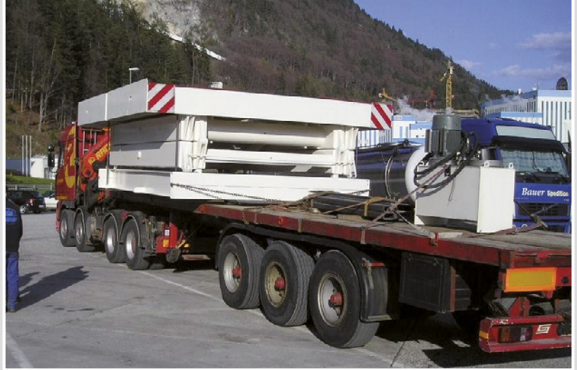
Capacity: 10,000 kg platform size: 5,000 mm x 4,400 mm stroke: 7,500 mm (special transport, wide load)
