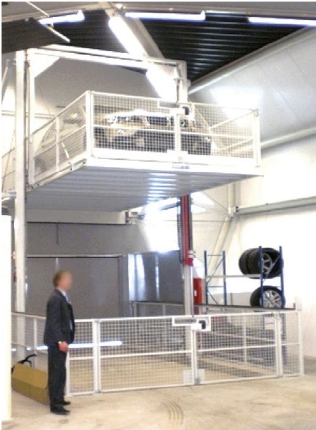
2-column car lifter, capacity: 2.5 t, effective stroke: 3.64 m
