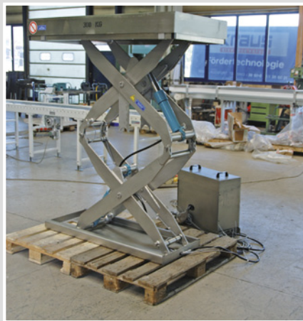
Capacity: 300 kg Stroke 1625 mm Stainless steel finish
