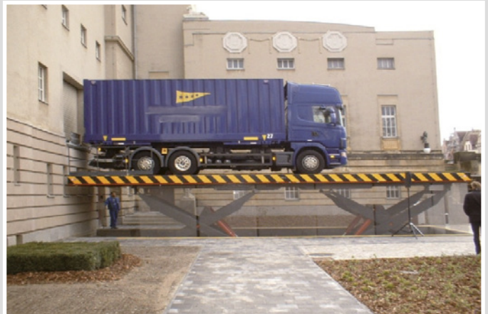
Capacity: 16.000 kg, Stroke 2.850 mm Carriage with geared motor
