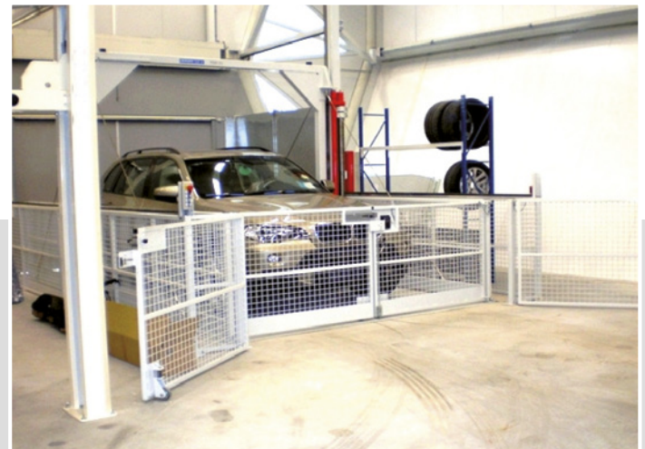
2-column car lifter, capacity: 2.5 t, effective stroke: 3.64 m
