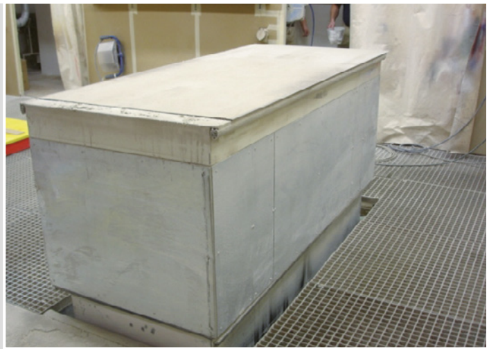
Capacity 1.000 kg, Plattform 1.980 x 980 mm, Hub 1.200 mm Use in spray booth, explosion-proof design Telescopic aprons, rubber switch-off rail
