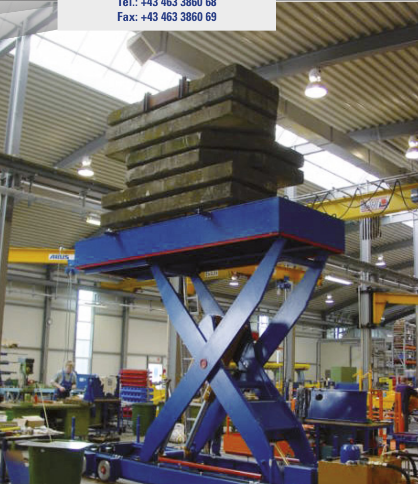
Capacity: 16.000 kg, Stroke 2.850 mm Carriage with geared motor
